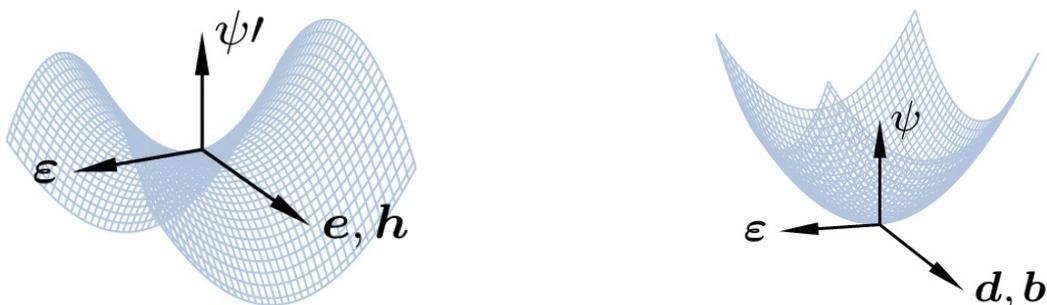
Fig. 1: Convex-concave and convex energetic functionals (thermodynamic potentials) related to minimization and saddle-point problems in electro-magneto-mechanics, adopted from [17].
