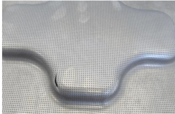
Fig. 3: Macroscopic crack initiation experimentally observed at the end of the cross section deep drawing of the DP1000 sheet [28].
